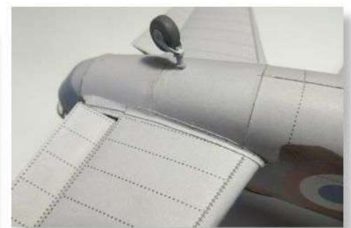
Noter le raccord karman aile/fuselage
