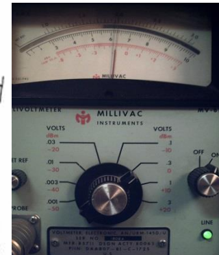
+ 0 dBm OUT 3.5 Mhz calibrated with 1 db loss of instrument's Head
