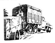
Radio Set AN/GRC-26 is a Mobile Selfcontained Radio Teletypewriter, Voice-CW Communications Center which can be operated in motion or stationary. The principal components are: BC-610 Radio Transmitter-2-18 mc-400W see page 9. R-388/JRR Radio Receivers. 5-30.5 see page 3. PE-95 Power Plant see page 32.
