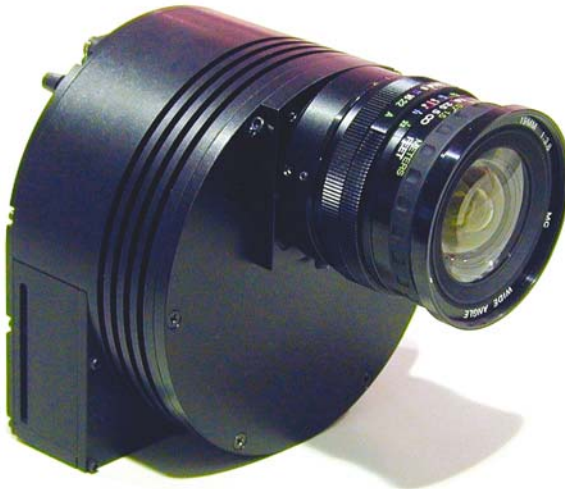
Figure 1.1. An SBIG ST7-MXE CCD camera. In this case it is shown fitted with a standard camera lens. The ST7 camera has been around for some years, but upgrades to the chip sensitivity and the connection type to the computer – in this case USB – mean this remains a popular camera. Image credit: Santa Barbara Instruments Group.
