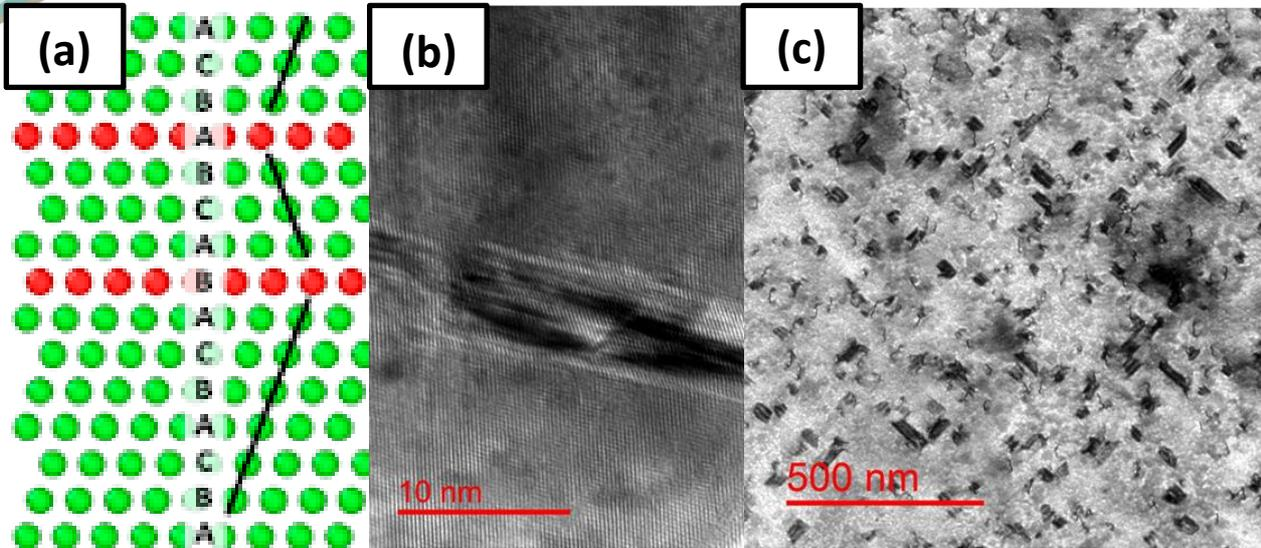
**Figure 1:** (a) Schematic of a twin. In the matrix, the atomic planes are in the order ABCABC; in the twin (bordered with the red planes) the order is reversed; image from S. Karewar et al, Acta Mater, 142 (2018) 71.
