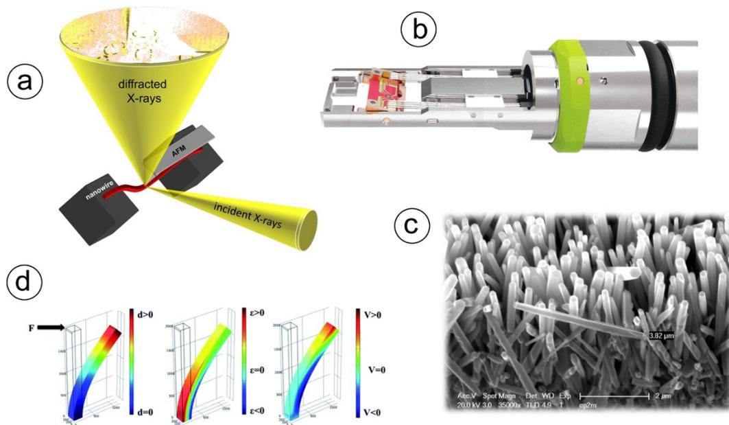
**Fig.1.** (a) Schematic representation of the bending experiment under X-ray beam. (b) Head of the in situ biasing TEM sample holder. (c) Scanning electron microscope image of ZnO nanowires. (d) Examples of finite element calculations of nanowires submitted to a bending mechanical stress.
