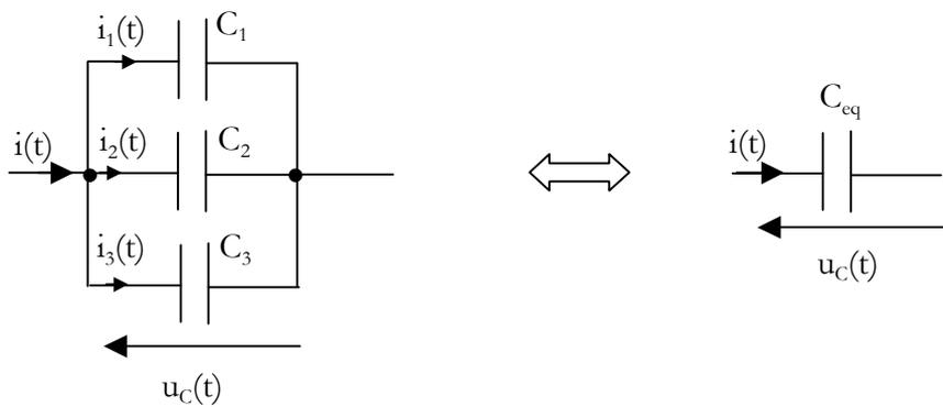
On a :  $q_1 = C_1 u_c$      $q_2 = C_2 u_c$      $q_3 = C_3 u_c$
