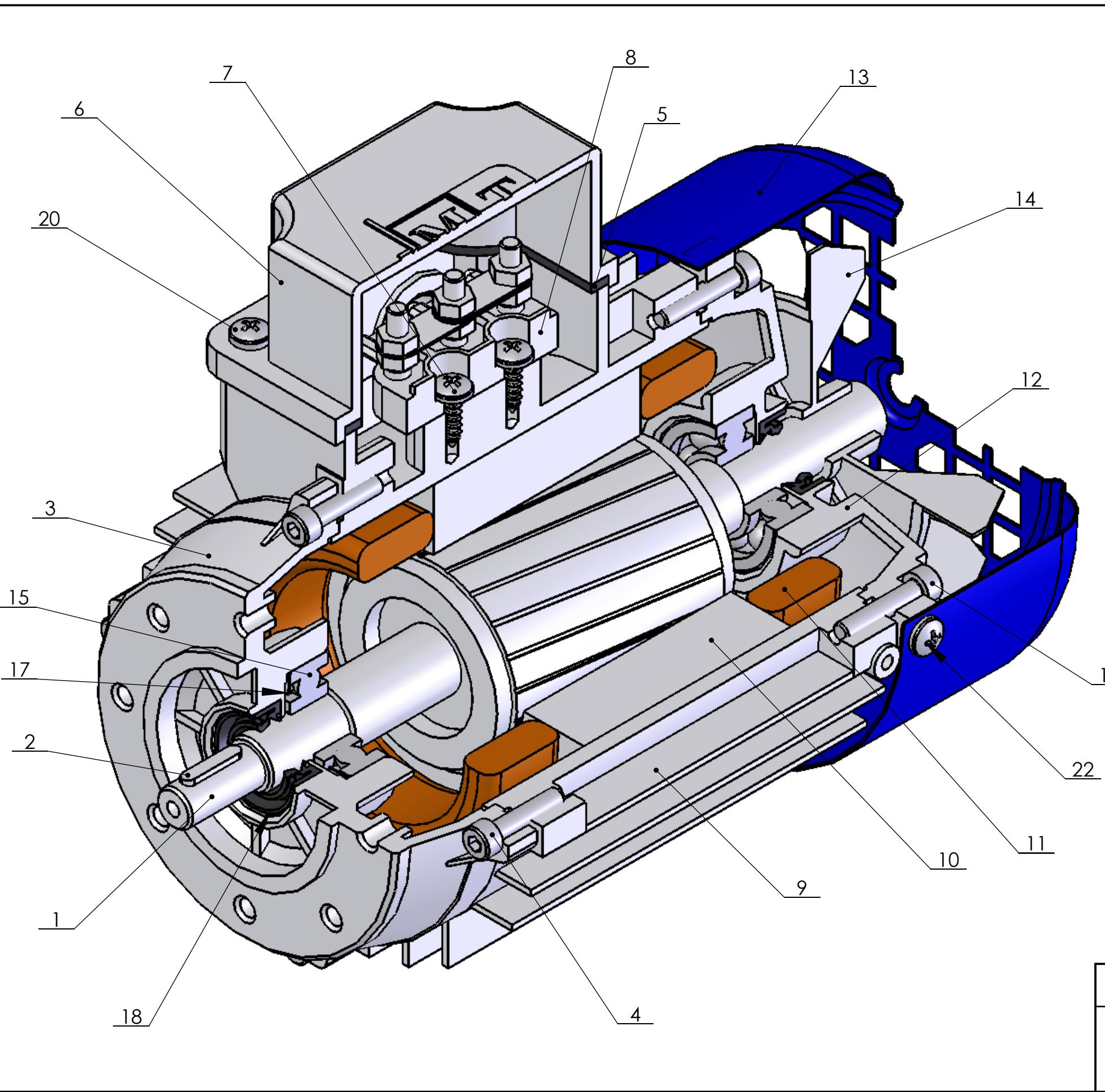
The diagram illustrates the exploded view of a 90W asynchronous motor. Various parts are labeled with numbers from 1 to 22, which correspond to the items listed in the bill of materials table.
